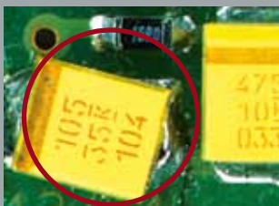
Defective placement, Tantalum capacitor
