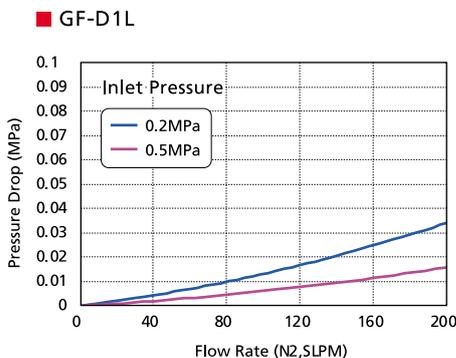
※The flow performance in case of 316L stainless steel gasket material is equal to the case of standard Ni gaskets.
